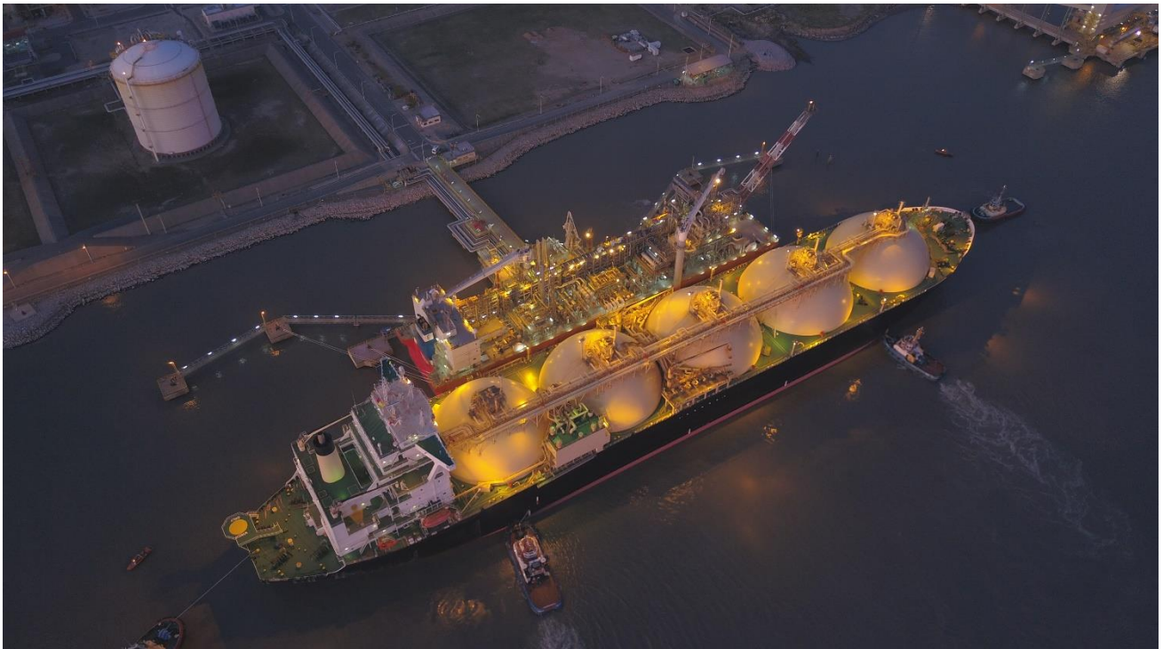
TANGO FLNG moored in Bahia Blanca (Argentina) receiving the cool-down cargo as part of the commissioning
