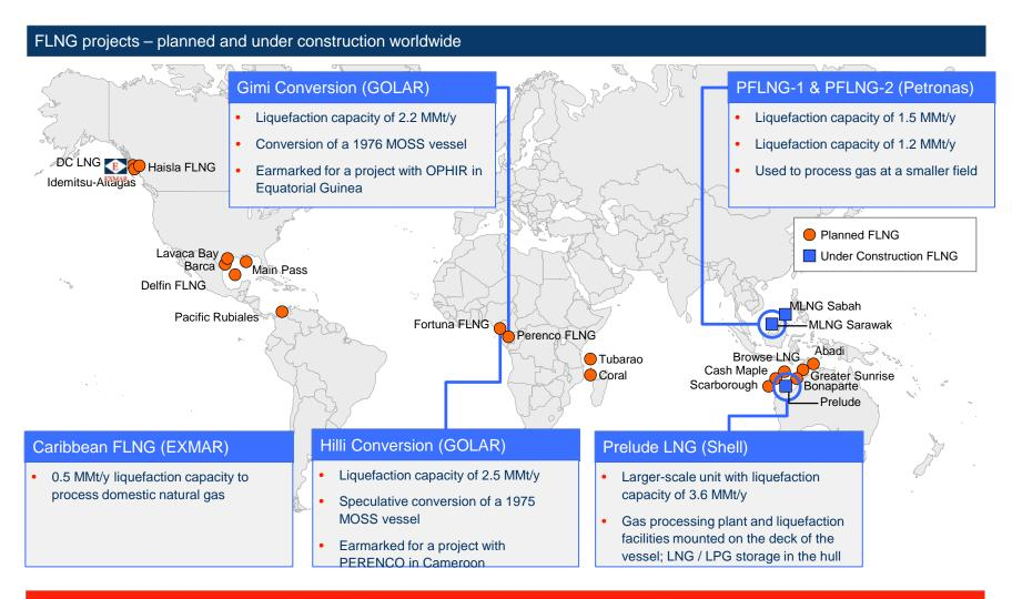
The FLNG solution provides an attractive and efficient alternative to traditional liquefaction
